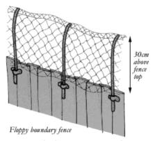
Figure 2. Diagram of a floppy boundary fence
