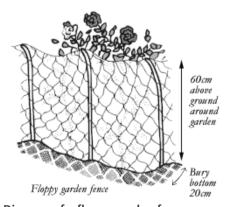
Figure 3. Diagram of a floppy garden fence.
